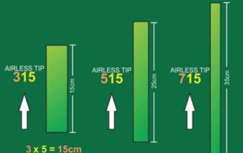
Multiply the first number by 5 and discover the fan spread in cm
