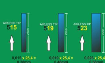
Add two zeros and multiply the last two numbers by 25,4 to know the size of the hole in mm
